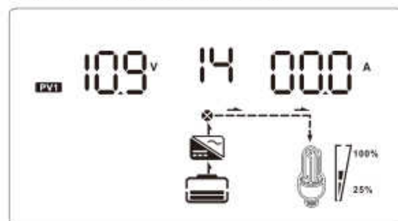
Page 14) PV1 voltage & PV1 current
