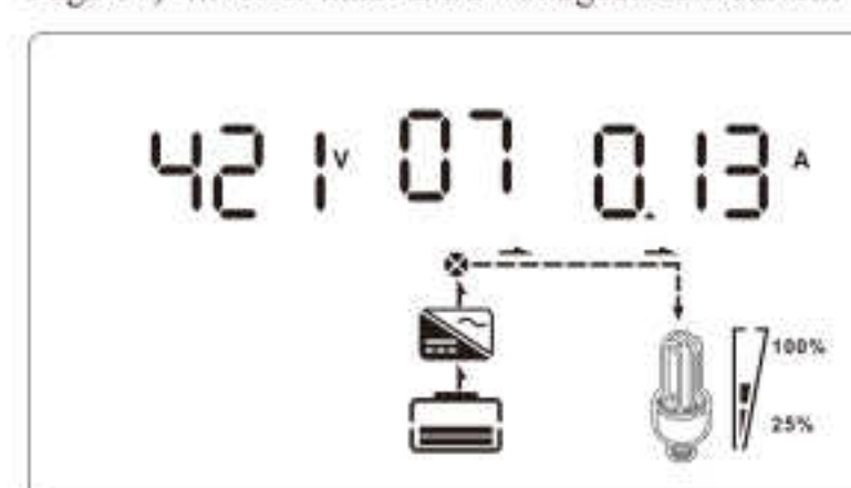
Page 07) Inverter inner BUS voltage & BUS current
