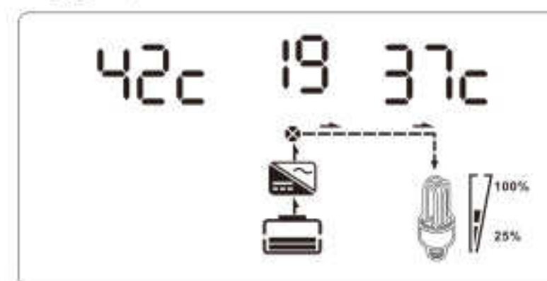
Page 19) Inverter Internal MPPT Heat Sink Temperature and Inverter Heat Sink Temperature (Note: This data for 3.3KW models is displayed on page 17)
