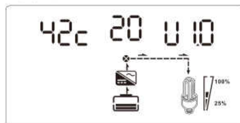
Page 20) Inverter Internal DC/DC Heat Sink Temperature and Software Version Number (Note: This data for 3.3KW models is displayed on page 18)
